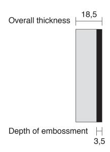
Besides the allowance of +/-0,3 mm of the total area thickness referring to the highest point there are minor differences in the thickness of the embossment - about 3,5 mm due to the natural design specifications.
